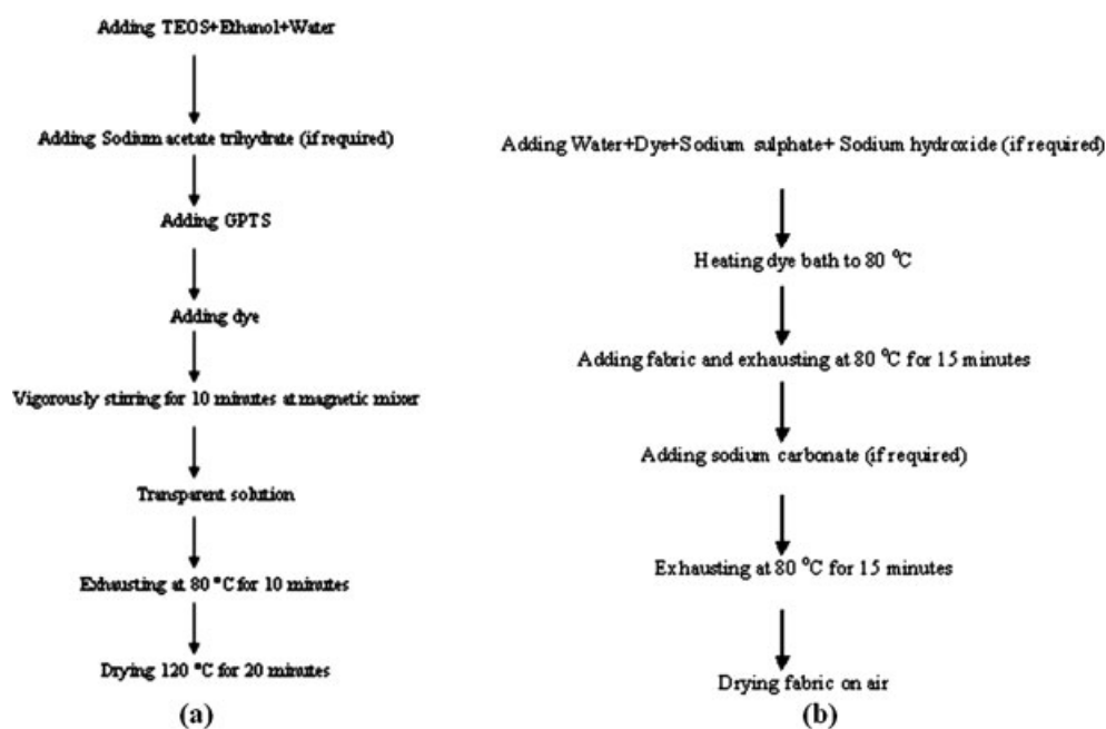
Figure 4 Flow charts of dyeing with (a) sol-gel process, (b) exhausting process.
